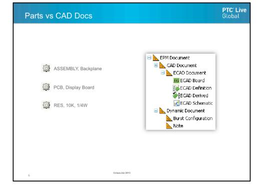
WTParts are objects to build product structures. They are associated with any object type in Windchill and do not contain CAD Documents objects, but reference the CAD documents. WTParts can also reference each other in a hierarchy called the product structure. They are symbolized in Windchill by a gear icon.
